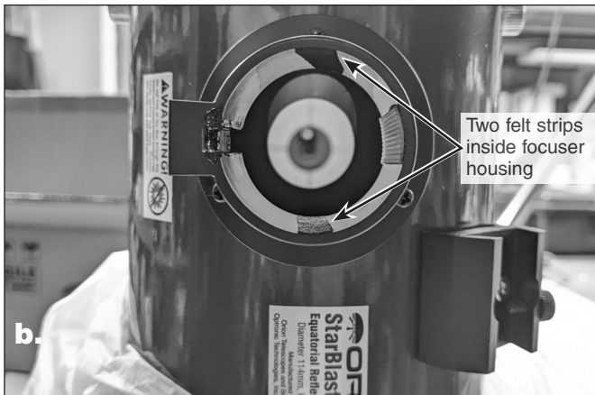
Figure 4a & 4b. Next we will apply the two felt strips on the inside of the focuser housing. Peel back the felt to reveal the adhesive and press gently to adhere to the inside. You will want to place them on opposite sides. Placement of the strips does not have to be precise – as long as the two strips are roughly facing each other the tube will be stabilized in the housing.
