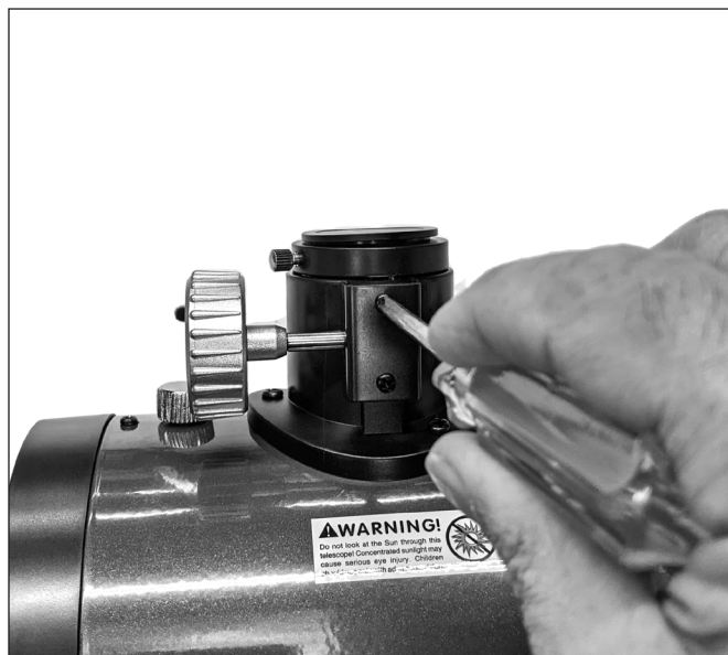
Figure 1. Remove the cover plate that holds the focus knob shaft assembly to the rack and pinion focuser by removing the two Phillips-head screws
